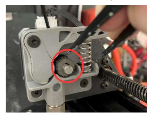
2. Clean up the residue of the filament on the gear. Clean with a pinch.
